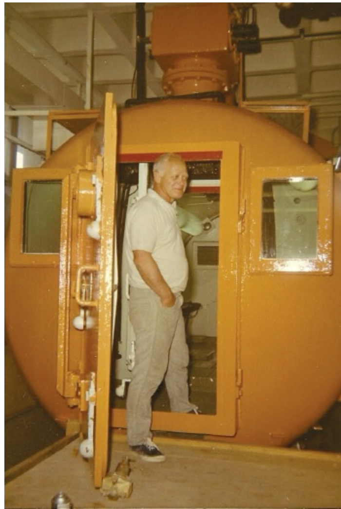
Figure 0.3 Dr. Steven Horvath standing in front of an environmental chamber designed to simulate high-altitude
